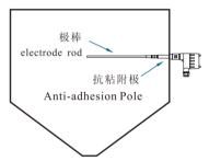
请注意不要让保护极缩在立管里面 Please do not let the protective electrode shrink in the pipe riser.
